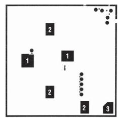
120mils × 121mils Backside metal: Alloyed gold layer Backside potential: substrate to Pad 2
